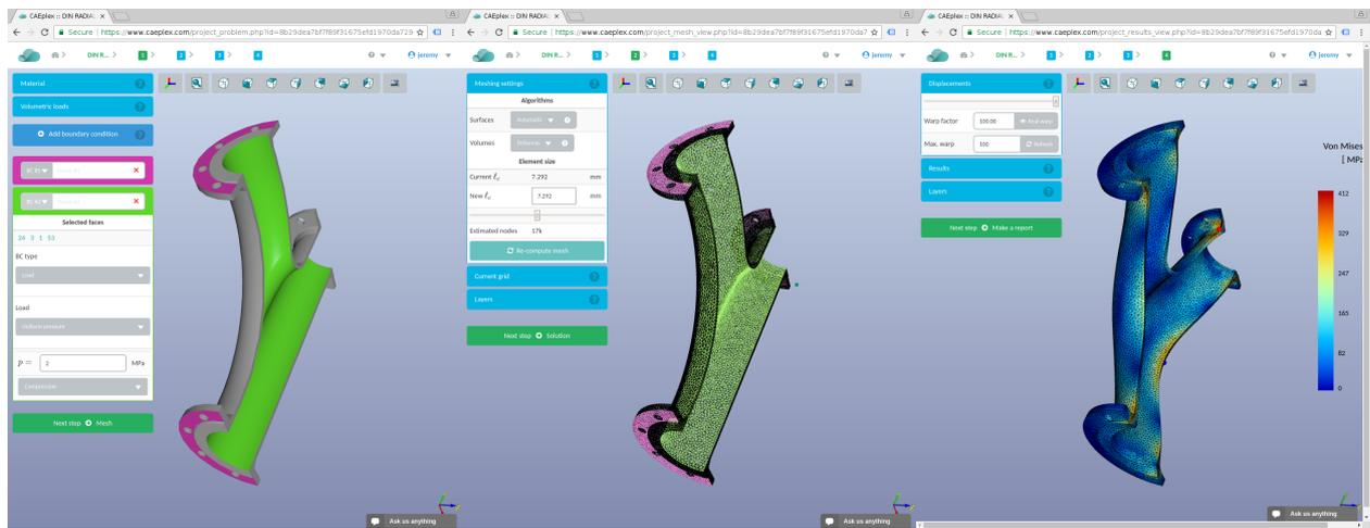
Figure 10: Fino and Gmsh running as a back-ends on the cloud for the web-based front-end CAEplex at caeplex.com
