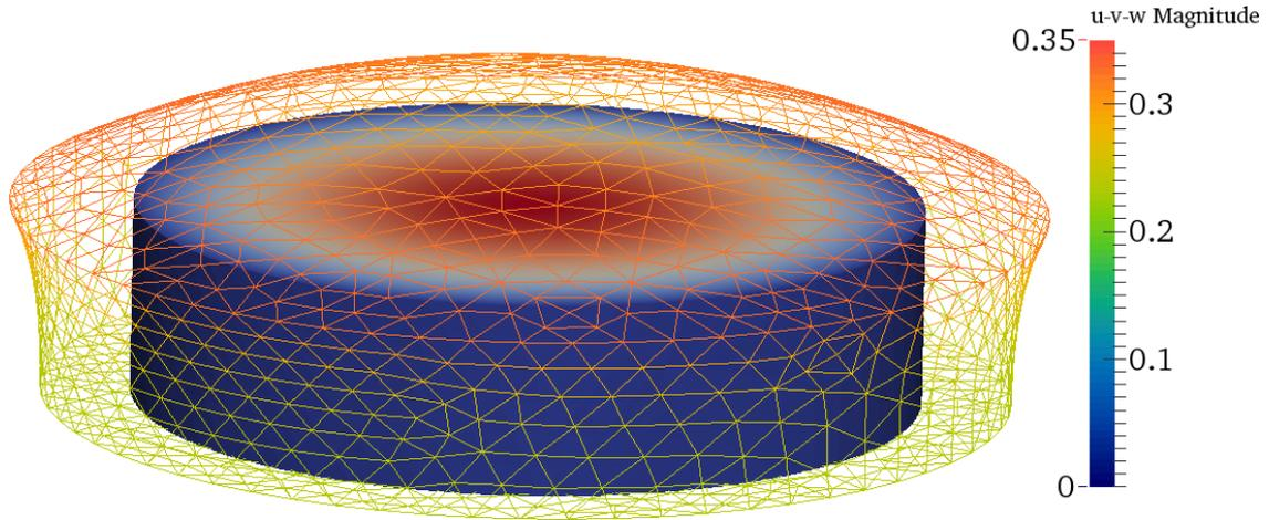
Figure 2: Illustration of the solution for  $h/b = 0.5$  and  $\nu = 0.333$  obtained by `finio` by postprocessing the VTK file it generates with `Paraview`.
