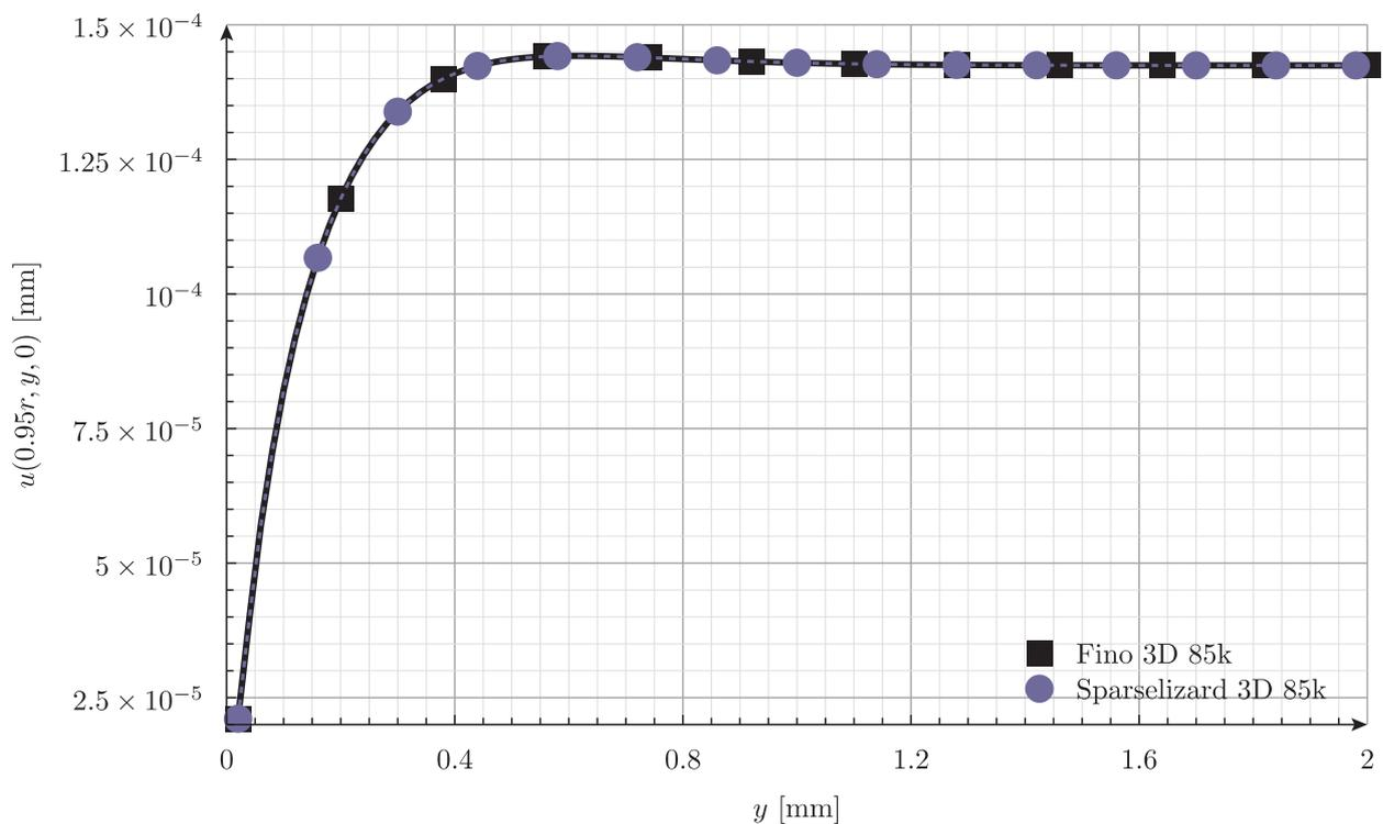
Figure 5: Horizontal displacement profile at  $x = 0.95 \cdot r$  and  $z = 0$  as a function of  $y$  computed by Fino and Sparselizard 3D with 85k nodes
