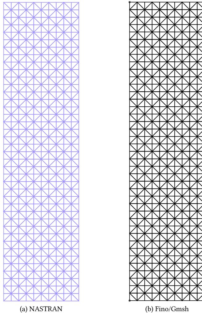
Figure 8: Axi-symmetric meshes with 1701 nodes each
