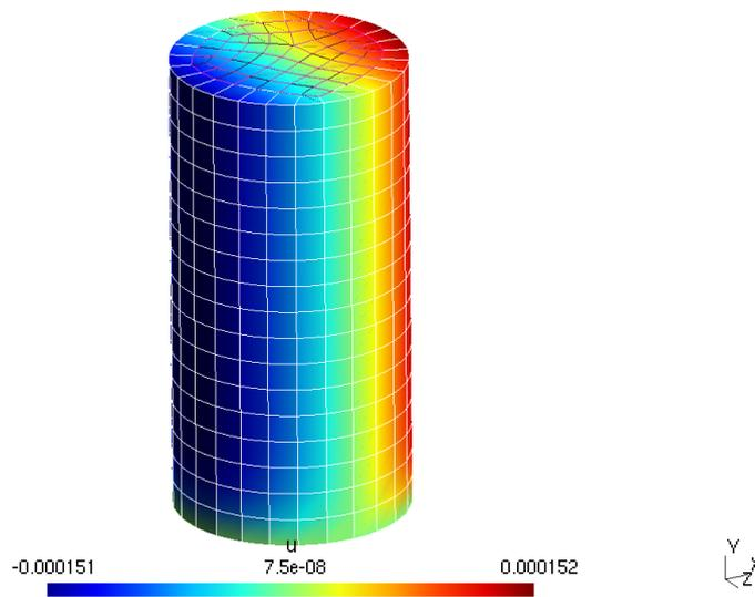
Figure 10: ANSYS solution to the 3D problem with 6.4k nodes using 20-node hexahedra
